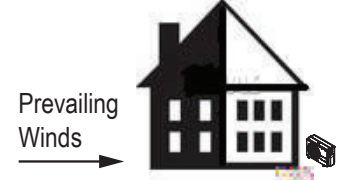
Figure 18: Leeward Side of the Building.
