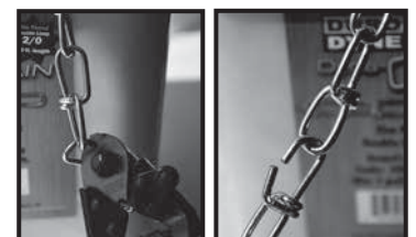
Cut with Duro Dyne Cable Cutter DTWRCL or DTRWC14
