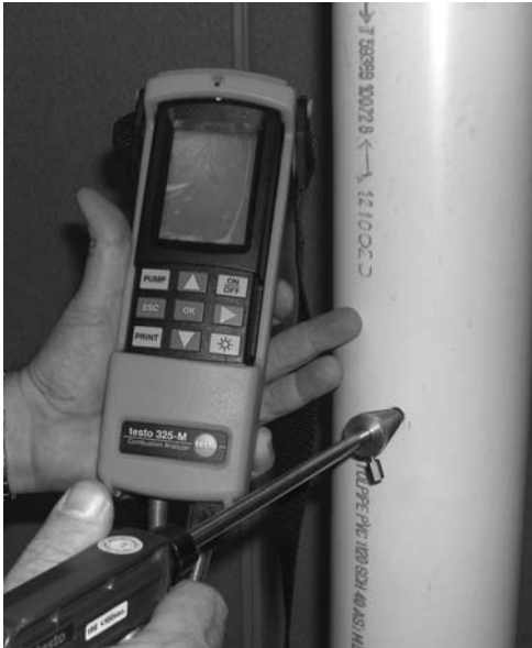
Figure 9.2: Insert Analyzer Test Probe into Test Port
