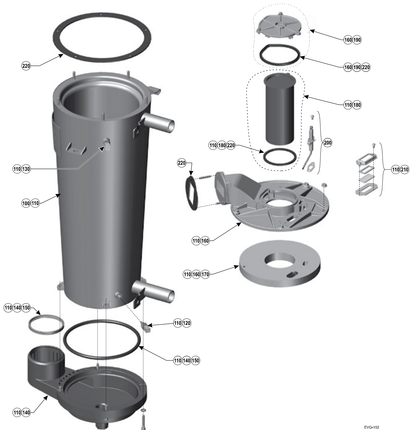
Figure 111 Heat exchanger assembly EVG 155 (see Figure 110 , page 126 for part numbers)
