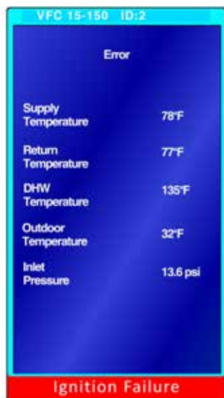
Error displayed after testing ignition safety shut off
