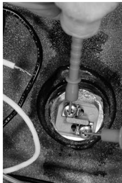
Figure 20. Element Resistance (ohms) Test
