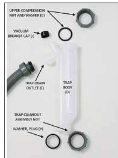
Condensate Trap, disassembled
