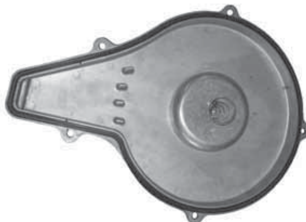
Figure 110 Heat exchanger cover plate removed
