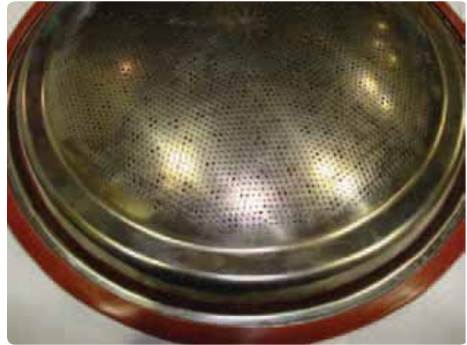
Figure 113 Inspecting exterior and cleaning the burner
